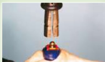
Wax-up with titanium sphere in position. Do not cover the "open" side of the base with wax.
