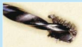
BROKEN SCREW BEING REMOVED
