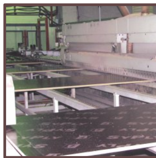
16. Cutting to size and edge profile trimming
