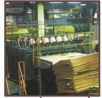
7. Patching and splicing
