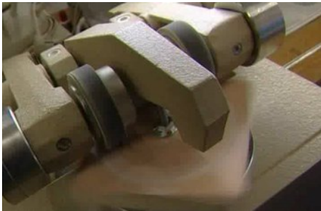
Abrasion resistance test (Taber-test)
