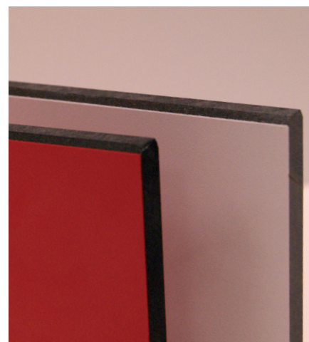
Wood fibre compact board with melamine coating and improved reaction to fire.
